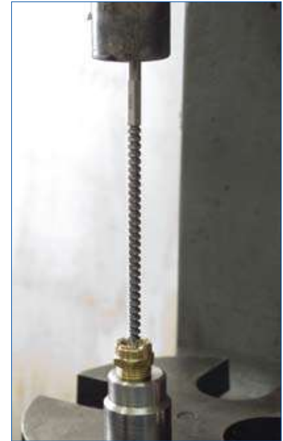
Pictured: A broaching operation using Hassay Savage push broaches.
